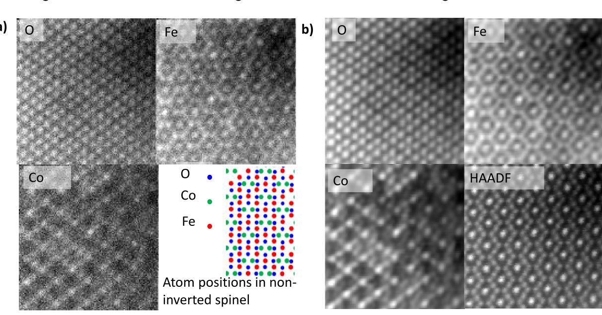
EELS elemental maps in the [110] direction after a) PCA and b) PCA+BM3D. Also shown are the atomic position projections in the non-inverted spinel and the simultaneous HAADF image. Some beam damage is visible in the top-right of the images.
